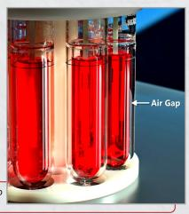
The patented SimAir® Test Cells, held in the (8) position SBT®+2 Carousel, utilize a unique air-gap between the test sample and the liquid bath medium to simulate the original air bath method.
