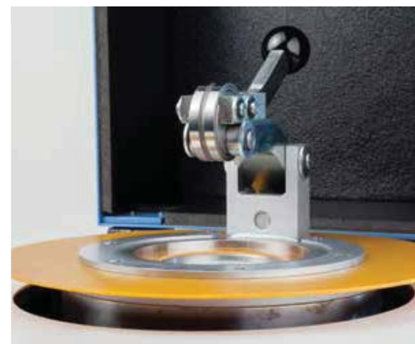
Manual clamping device with and without grinding vessel (50 ccm)
