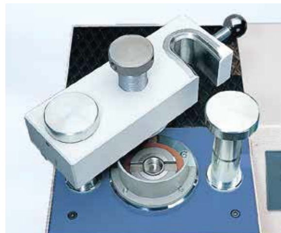
Swing-out cross-head for easy machine handling
