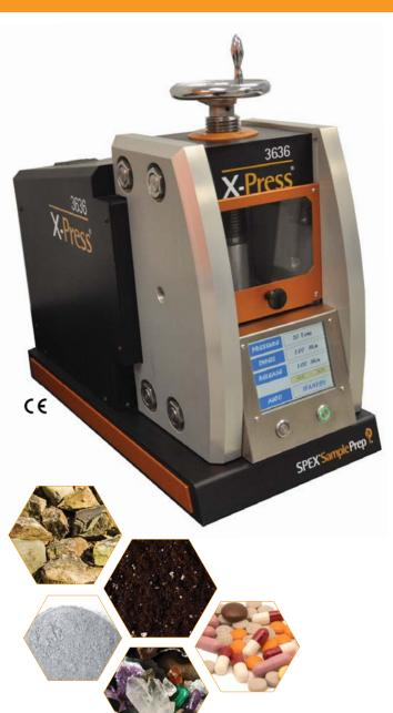
The 3636 X-Press® is a 35-ton (31.8 metric ton) hydraulic laboratory pellet press that is ideal for accurate and repetitive pressing of sample pellets for XRF and other analytical techniques.
