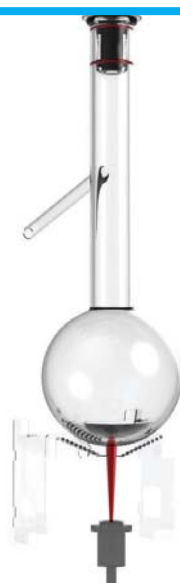
Optical Dry Point
