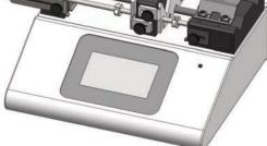
Large syringes can acheive full stroke length by repositioning the adjustable syringe holder.
