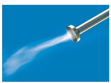
The QA40 Atomizer uses ultrasonic energy to generate a low-velocity, gentle spray. The sample can be precisely delivered to the target area. Overspray is virtually eliminated resulting in material savings. The atomizer can run continuously or be programmed to pulse on and off.
