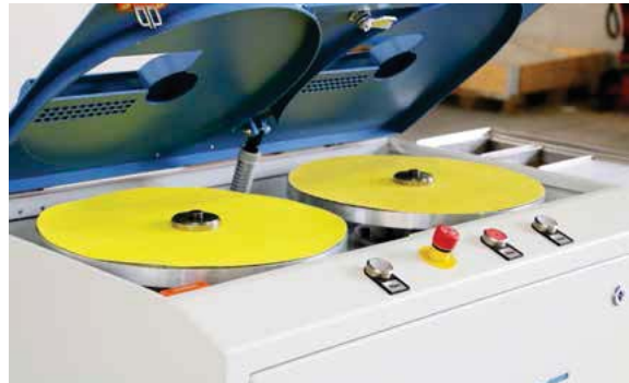
The HT 350 has two separately driven discs grinders.
