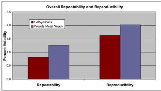
Data taken from the ASTM Test Monitoring Center (TMC) Round Robin study are shown in the adjacent graphs. The Selby-Noack has very good correlation to the Wood's Metal Noack with better overall precision.
