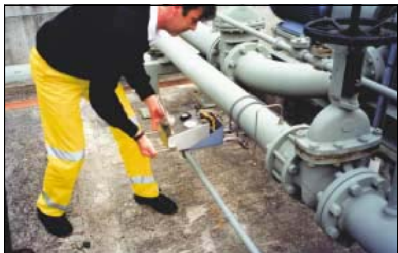
Permanently installed mounting tray and removeable Sampler
